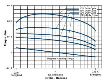
Graph 2 shows operation end-to-end. Note the high starting torque for high starting acceleration or for stopping the load by means of reverse voltage at the end of the stroke. If the device is used in a full stroke application, the load can be externally latched, detented, or biased to either end of stroke.
