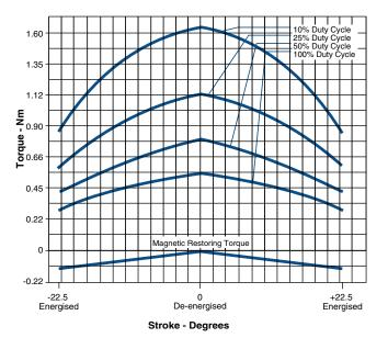
Graph 1 shows three position operation. In any mode, the armature seeks centre of stroke at zero power.
