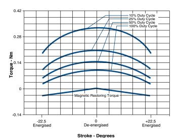
Graph 1 shows three position operation. In any mode, the armature seeks centre of stroke at zero power. Applying a positive or negative voltage causes the shaft to rotate clockwise or counter clockwise. When power is removed, the restoring torque is applied to the load, or alternatively, the shaft can be driven to centre under power.
