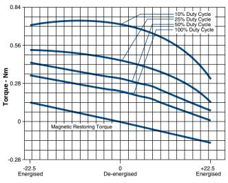
Graph 2 shows operation end-to-end. Note the high starting torque for high starting acceleration or for stopping the load by means of reverse voltage at the end of the stroke. If the device is used in a full stroke application, the load can be externally latched, detented, or biased to either end of stroke.
