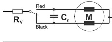
Series circuit 230V (for motors with resistance  $R_{20} = 12600 \Omega$ )
