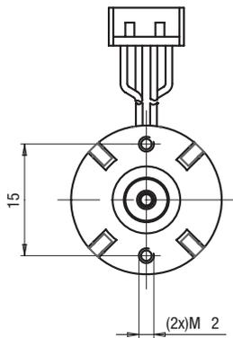
Use bolts with thread length 4mm max. Screw in torque 10cNm max.
