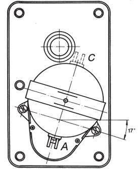
Lead outlet (A = standard position)
