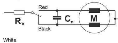
Series circuit 230V (for motors with resistance  $R_{20} = 11800 \Omega$ )
