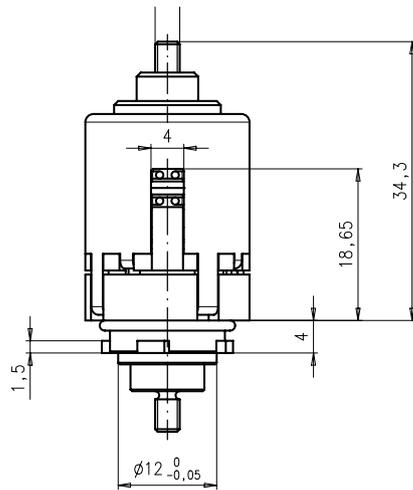
Connecting dimensions of direct bayonet mount
