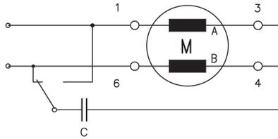
Parallel circuit 230 V (only for connector N) with 110 V motor and capacitor  $C_V$
