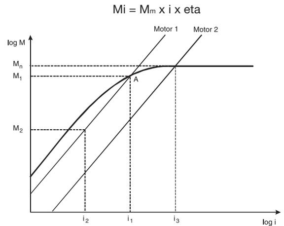
Example 1: The application of Motor 1 combined with a gearbox of ratio  $i_1$  leads to an output torque  $M_1$  at point A. The gearbox can transmit this torque, meeting its lifetime.
