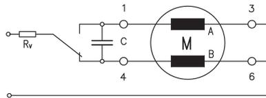
Parallel circuit 230 V (only for lead wire versions) with 110 V motor and capacitor  $C_V$
