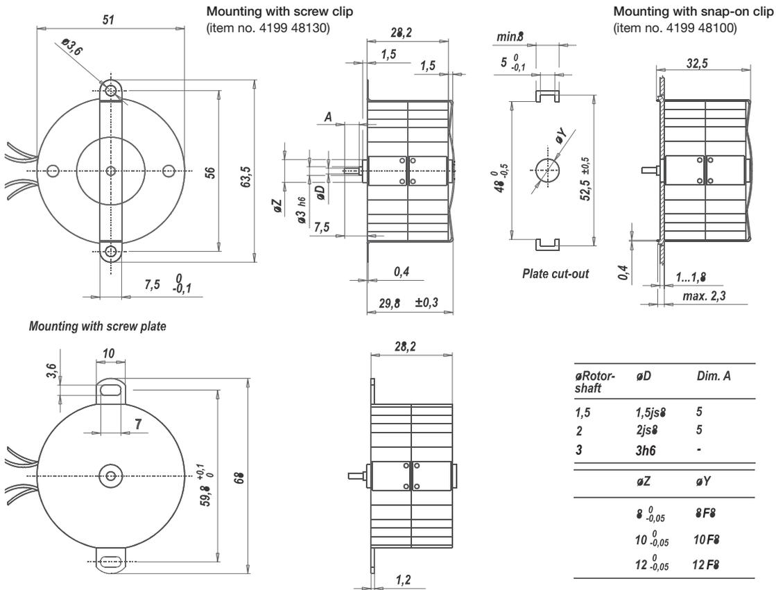
Lead wires: AWG 22 (0.34 mm<sup>2</sup>), insulation diameter  $\varnothing 1.72 \pm 0.08$  mm, 6 mm stripped
