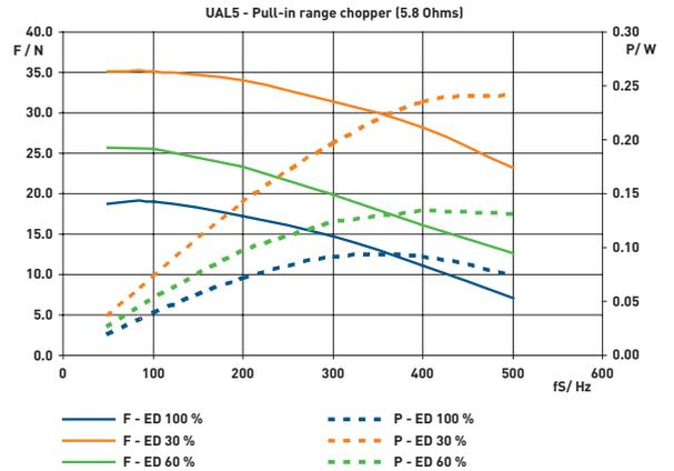
100% duty cycle: max. current per phase 300 mA
