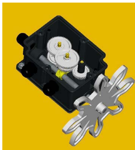
Picture 4.: Rendering of gear wheel inner the plastic box
