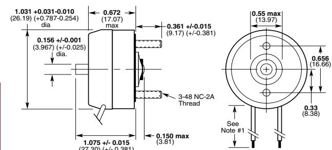
Armature Cover Configuration — Double Shaft
