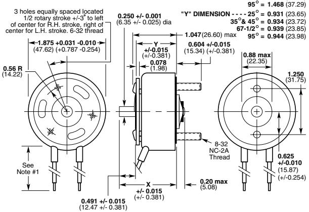
Armature Cover Configuration — Base End Shaft
