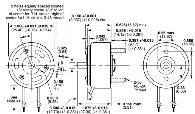
Armature Cover Configuration — Base End Shaft
