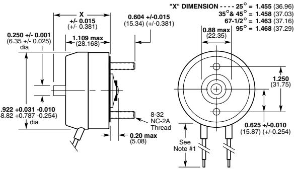
Armature Cover Configuration — Double Shaft
